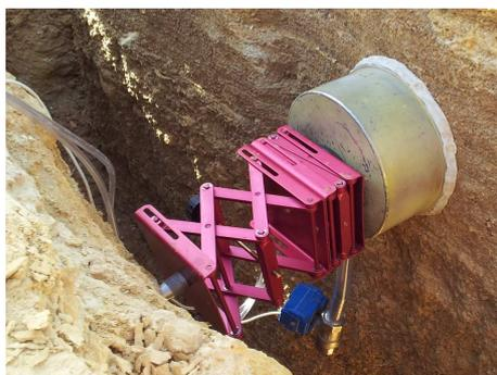
Figure 6. Exhalation measurement on a crack wall
